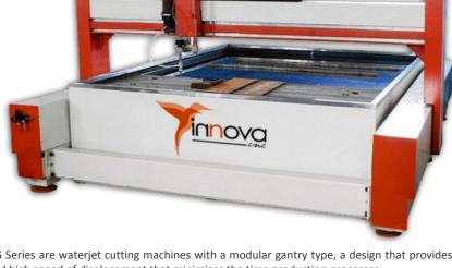
Wassercut SG Series are waterjet cutting machines with a modular gantry type, a design that provides great structural robustness and high speed of displacement that minimizes the time production processes.
